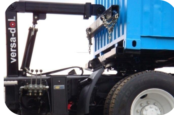
container is secured to the turntable via ISO twist locks
