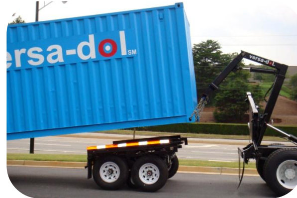
container's far-end is grounded, dolly retrieved from beneath the container
