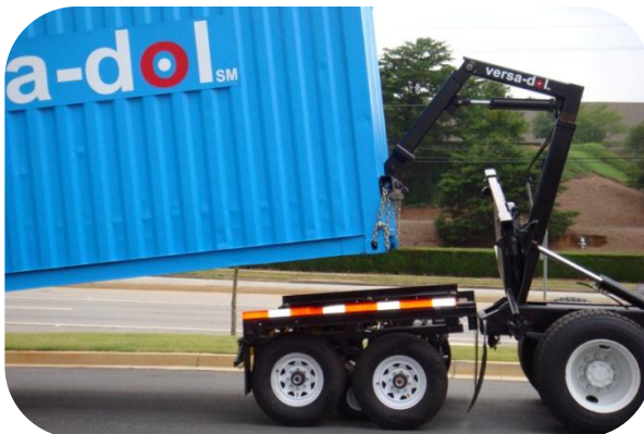
road tractor and dolly simultaneously track forward as container is lowered
