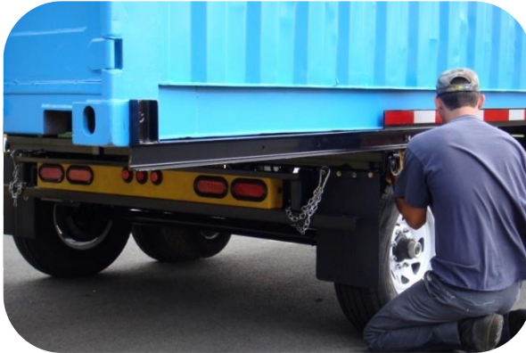
dolly is secured to the container with locking bars and DOT approved tie-down straps
